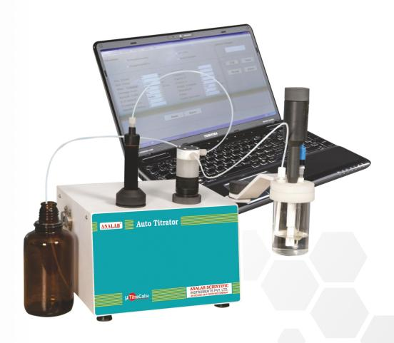
Basic Unit consist of Combined Glass Electrode with suitable connector, Rod Stirrer, Titration Vessel holders, Titration Vessels, 20ml Burette, Valve Jet assembly, Teflon Tubing with Connector, Stand, Standard Software (without computer), Communication Cable, Operational & Instruction Manual with SOP, Calibration Test Certificate (Without Traceability Document) and Warranty Card.
