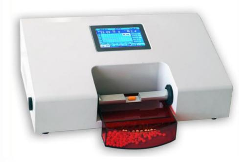
Tablet hardness tester adopts high-performance, embedded ARM'Cortex-M3' core processor, combined with the highest-performance mechanical A/D module chip to ensure high-speed acquisition and lossless processing of measurement data. Provide professional users with reliable and accurate measurement results.
