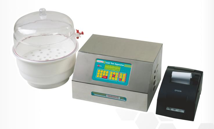
Supplied with Vacuum Pump (Inbuilt with System), Silicon Tube, Power Cord, Operational & Instruction Manual with SOP, Calibration Test Certificate (Without Traceability Document) and Warranty Card.
