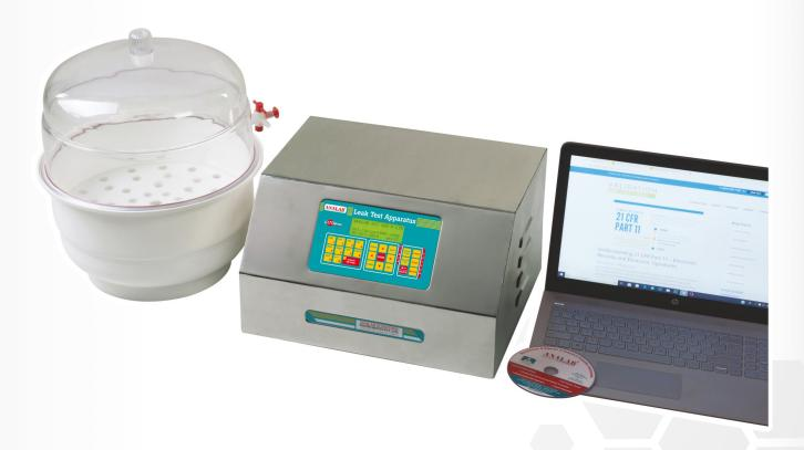
Supplied with Vacuum Pump (Inbuilt with System), Silicon Tube, ANALABsafe software, USB Interface Cable, Operational & Instruction Manual with SOP, Calibration Test Certificate (Without Traceability Document) and Warranty Card.
