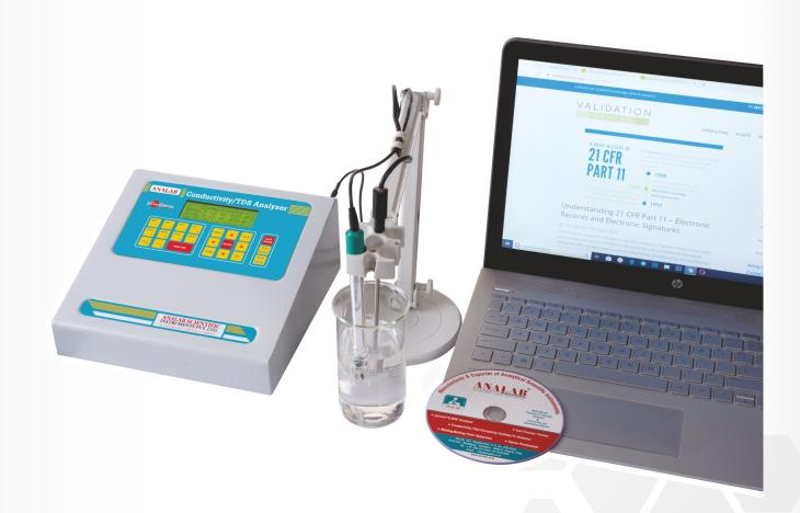
Supplied with Conductivity Cell K=1.0, Temperature Probe, Electrode Stand consists of Clamp, Base Plate & Rod, Dust Cover, DC Adaptor, ANALABsafe software, USB Interface Cable, Operational & Instruction Manual with SOP, Calibration Test Certificate (Without Traceability Document) and Warranty Card.
